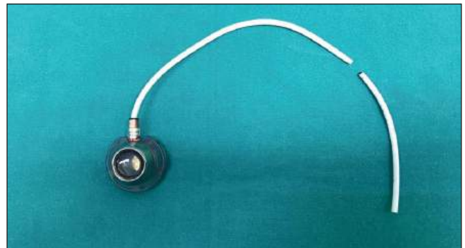
Figure 4. Teared TIVAD material reassembled after removal.
