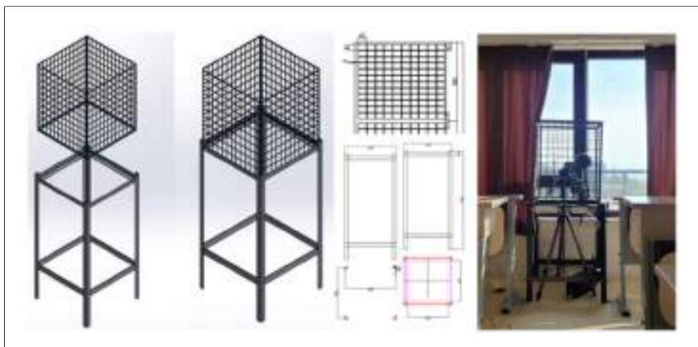
Figure 4. Protective enclosures for thermal comfort measurement devices.
